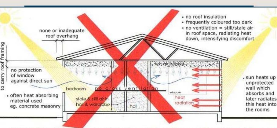
conventional cross section & construction method (roof trusses)
